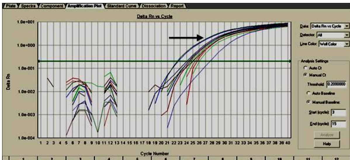
Figure 3: Proper Amplification Curve
