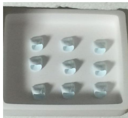
Figure 9. The teeth were sintered
