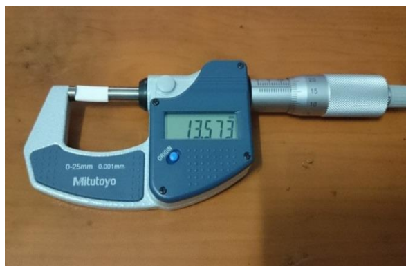
Figure 2. Dimension of specimen after sintering.
