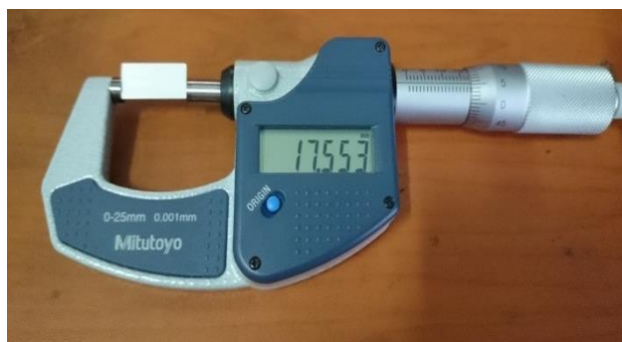
Figure 1. Dimension of specimen before sintering.
