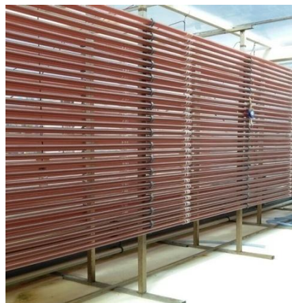
Figure1. The tubular photobioreactor system
