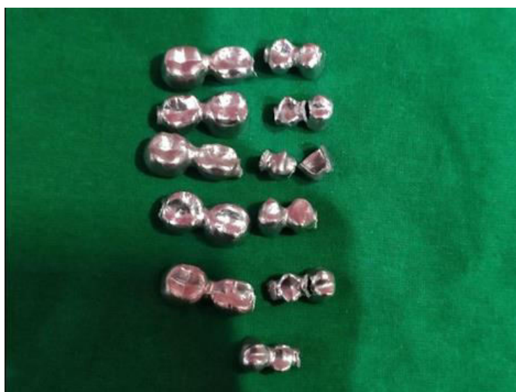
Figure 32: Group B - Resin Pattern Casting Fractured Samples with Comparative Higher Resistance
