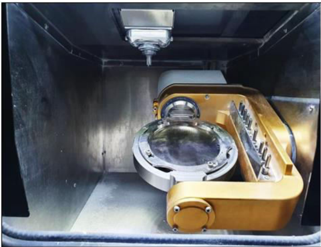
Figure 8: Co-Cr Blank in Milling Uni
