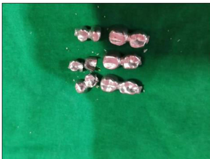
Figure 33: Group B - Resin Pattern Casting Fracture Samples with Comparative Lower Resistance
