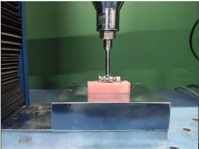
Figure 28: Load Applied on Centre of Connector Area
