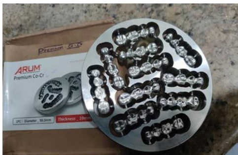
Figure 9: Milled Samples on Co-Cr Blank
