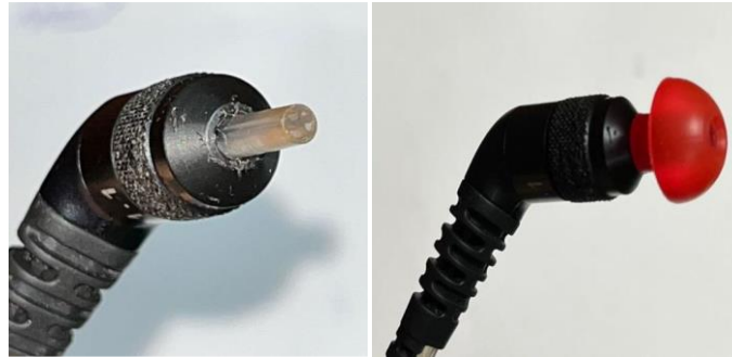
Fig 2: RIGHT: Soft rubber probe tip to create airtight seal in the ear canal, LEFT: Probe tip having 3 channels
